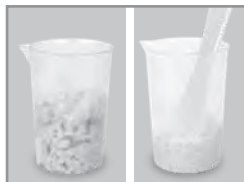
3. Fill the beaker with pulp up to the 250 mL line. Press down & flatten the pulp so its final height is between the 50-75 mL lines.
