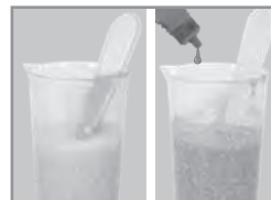
4. Add water to the beaker until contents are at the 250 mL line. Add ink drops to make desired color. Stir with the spatula until pulp slurry is uniformly thick & slightly lumpy.
