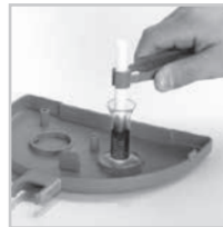
4. Using the tweezers, gently lower a core into the measuring tube. Allow core to sit until all ink is absorbed.
