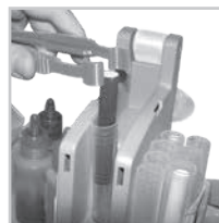
7. Push core down into barrel.
